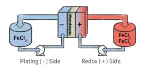
With the same electrolyte running on both the negative and positive sides, there is no risk of cross contamination.
